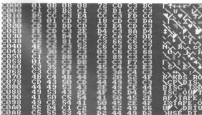
Erm... This is, erm, what exactly? Oh yeah - it's a hexadecimal representation of the first few bytes of the ROMDOS ROM. If you look closely, you can see the ASCII characters of the commands, complete with last bit set on the last character.
